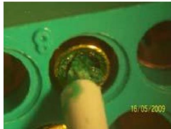
Corrosion product on cables from flux residue
